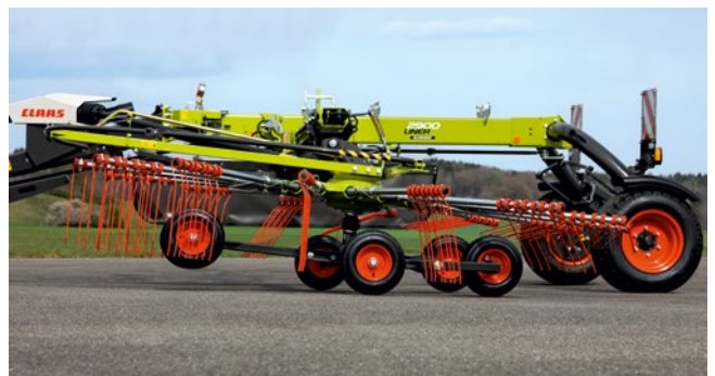
For healthy soil: During lifting and lowering the rear wheels touch down before the front. The rotor behaves like a plane taking off and landing, called the Jet Effect.
