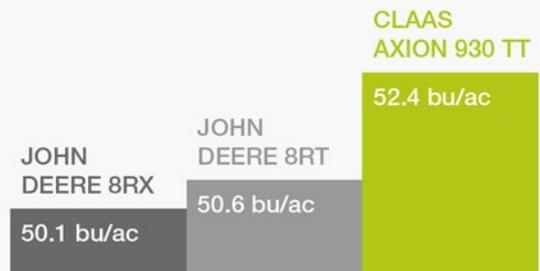
**Why?** Even during tight headland turns, the front wheels pull the rear tracks smoothly so soil remains level with minimal berming or disturbance for evenly distributed ground pressure - ultimately increasing yield. Plus, standard on every AXION TERRA TRAC tractor, automatic brake assisted steering is integrated into the existing machine brakes for a seamless turning experience.
